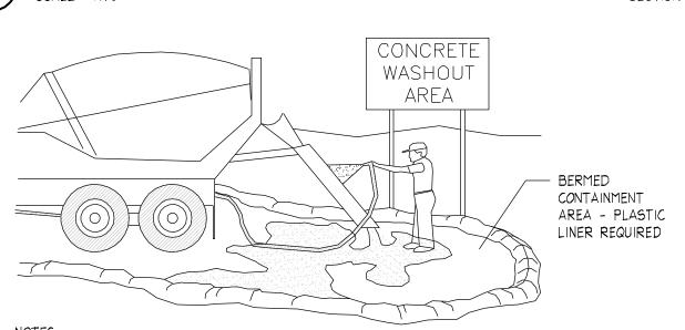
EXCESS AND WASTE CONCRETE SHALL NOT BE WASHED INTO THE STREET OR INTO A DRAINAGE SYSTEM.
