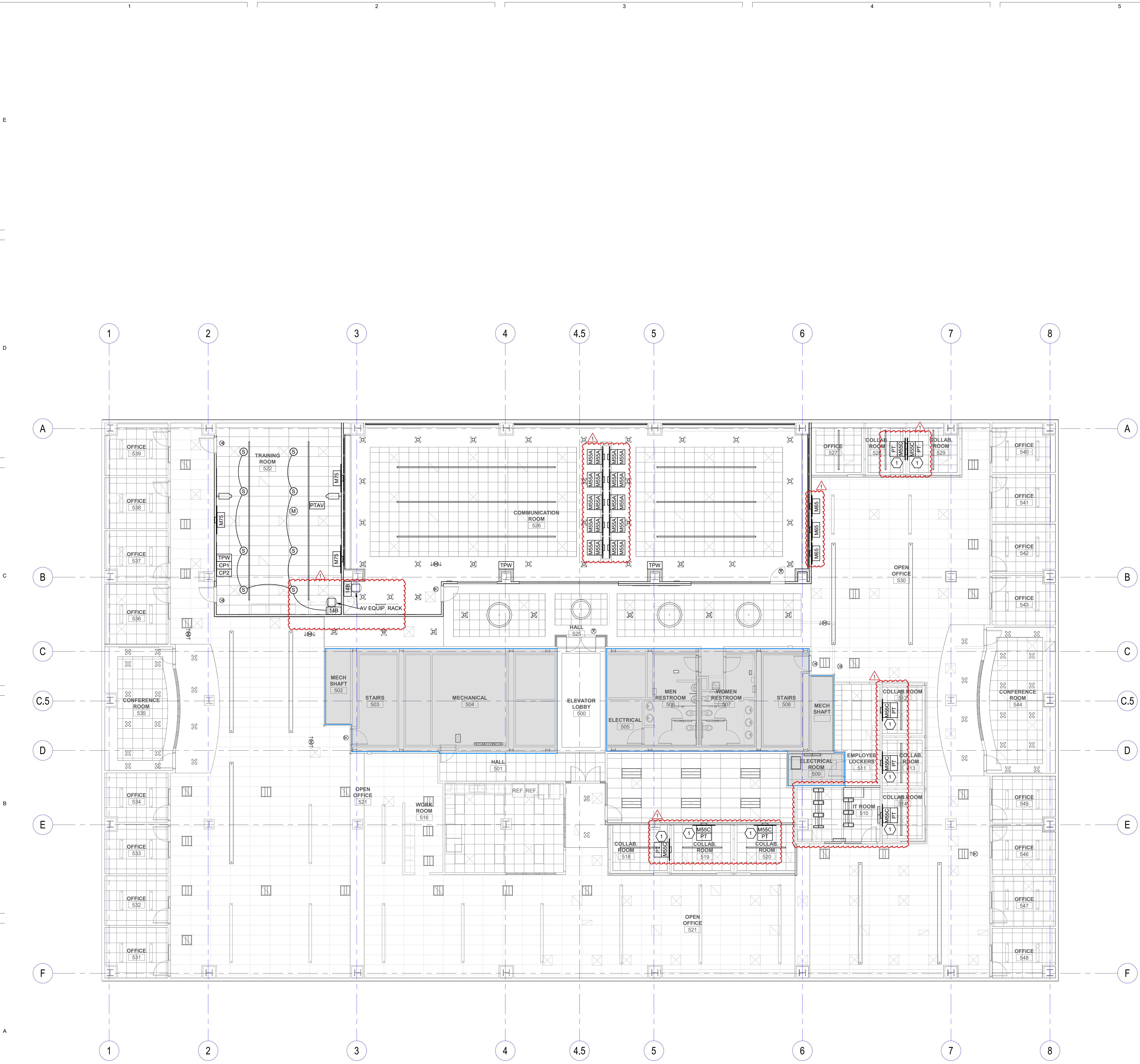
A1 LEVEL 5 AUDIO VISUAL ROUGH-IN PLAN SCALE: 1/8" = 1'-0"
