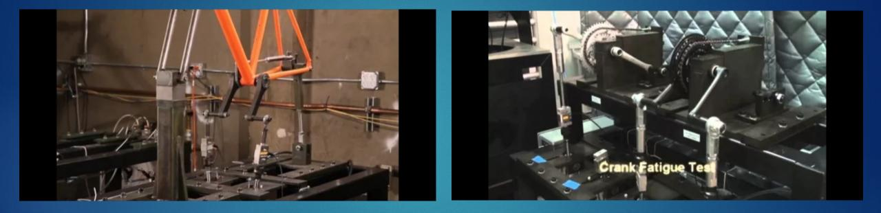
Frame fatigue test with pedaling forces: Lateral flexing of frame – no energy return <u>https://www.youtube.com/watch?v=8blo6O\_KIAs</u> Crank fatigue test with pedaling forces: Twisting of crank arms – no energy return <u>https://www.youtube.com/watch?v=7rZ1L6brkNE</u> Up to 1.6 % loss at 100 rpm, more at lower rpm
