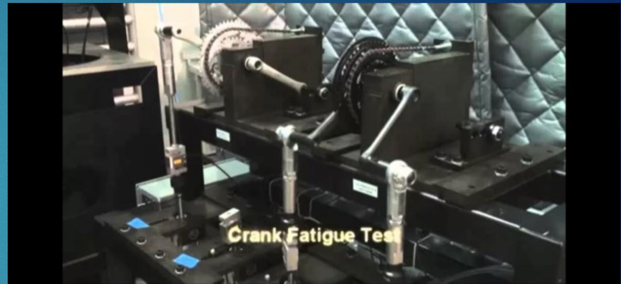
Crank fatigue test with pedaling forces:
