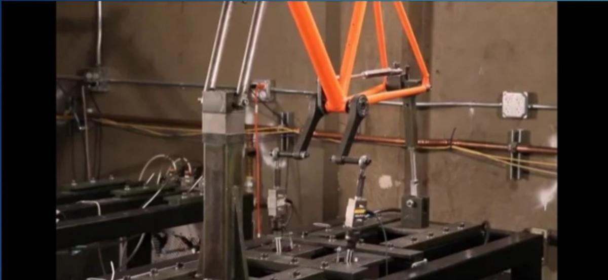
Frame fatigue test with pedaling forces:
