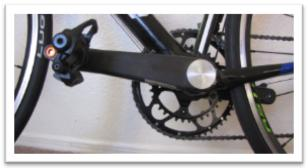
Lightweight Carbon based IMPACT Drivetrain Crankset Prototype
