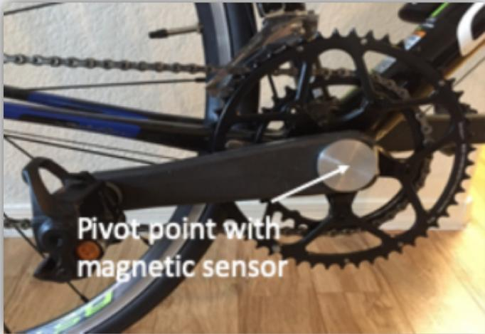
Source: Location of magnetic rotary sensor between crank arm and spindle
