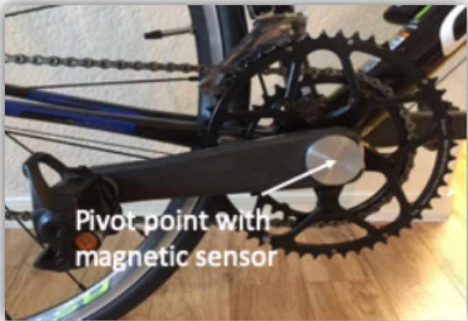
Source: Location of magnetic rotary sensor between crank arm and spindle
