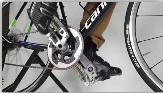
Source: Aluminum proof of concept crank set in action
