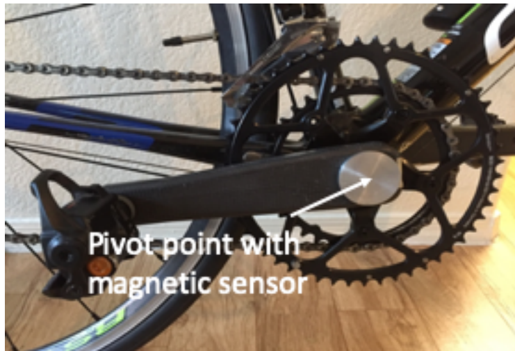
Figure 3. Location of magnetic rotary sensor between crank arm and spindle
