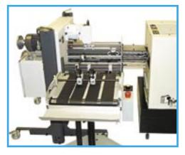
The K20 Knife Folder shown at the end of an in-line finishing system to guarter-fold booklets for lower cost mailing applications.
