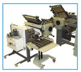
The K20 Knife Folder shown with the Baum 2020 Parallel and 8-page folder with Baum 20 hang-on delivery stacker and mobile stacker kit. The K20 can be used to complete signatures, double gatefolds and more.
