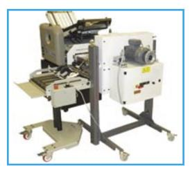
The K20 Knife Folder shown with the Baum 714XLT tabletop folder and optional Baum 20 delivery stacker with mobile kit. The 714XLT makes an excellent feeder for pre-folded sets when feeding the product spine edge first is required. The tabletop folder is also equipped with the high speed transfer table used with the Baum 714XLT 8-page folder.
