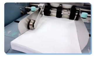
Standard **cross folding** unit for right-angle folds provides greater application possibilities.
