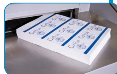
Low-friction work table and extra-large side tables help operators process large and/or heavy paper stacks with ease
