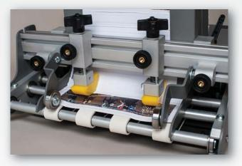
Buckle Separation<sup>™</sup>, another Straight Shooter innovation, easily separates documents without the jams common with traditional feeders. The R-14 comes with **three** independently adjustable separators... **Versatility!**
