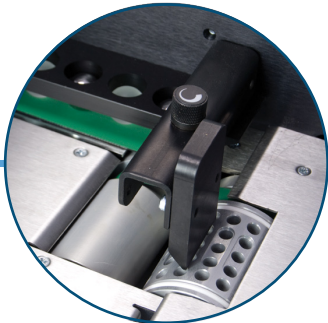
Powerful Air Suction Feed Table Handles coated and non-coated stock, in sizes up to 26.5” long
