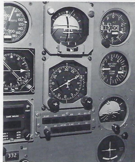
Sperry SPZ-500 autopilot, new flight director system, air data computer and displays, plus Sperry STARS radio altimeter. New autopilot controller for SPZ-500 is mounted on center console beneath throttles.
