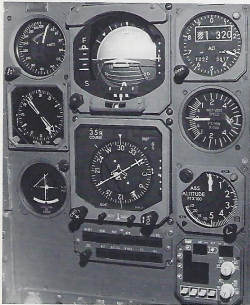
STANDARD IN CITATION --- Cessna Citation panel features new Sperry SPI-81 5-inch instruments on pilot's side and 4-inch STARS instruments on right. Citations from aircraft number 275 and subsequent are equipped with
