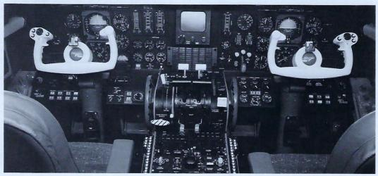
SOLID PERFORMER — All Sperry components in this Grumman Gulfstream II performed flawlessly during installation, checkout and flight test at Executive Aircraft Services, Redbird Airport, Dallas, where work was done. N903G, G-II serial 172, was delivered Mar. 19 and is based at Toledo (Ohio) Express Airport. Installation, first in a G-II involving a full SPI-80 flight director system, was
