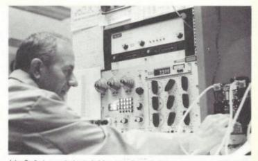
John Szallasi, an avionics technician, tests three air data computers on a HG180 Air Data Computer test station. The electro-static and climate control systems at the new location assure the maximum reliability of the repairs and tests.
