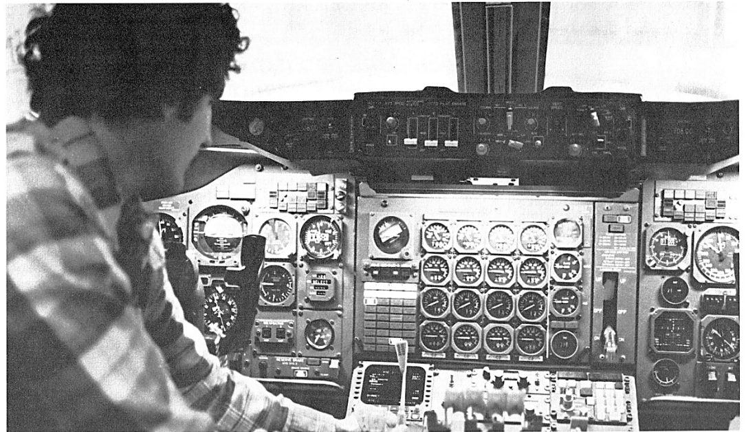
SPERRY PROJECT ENGINEER Curt Walters checks out Flight Management System aboard British Airways Boeing 747 before the system's first trans-Atlantic test flight. FMS control display unit is at upper left of center console, above Walters' left hand.
