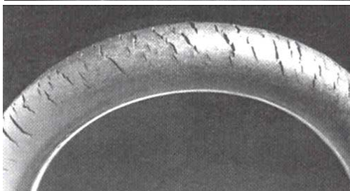
Ozone cracking in natural rubber tubing.
