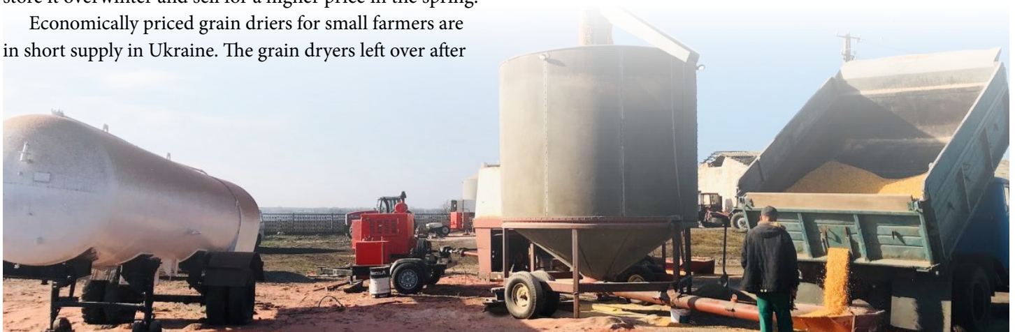
A farmer unloads corn into the grain dryer. The tanker at left has propane to dry the grain.
