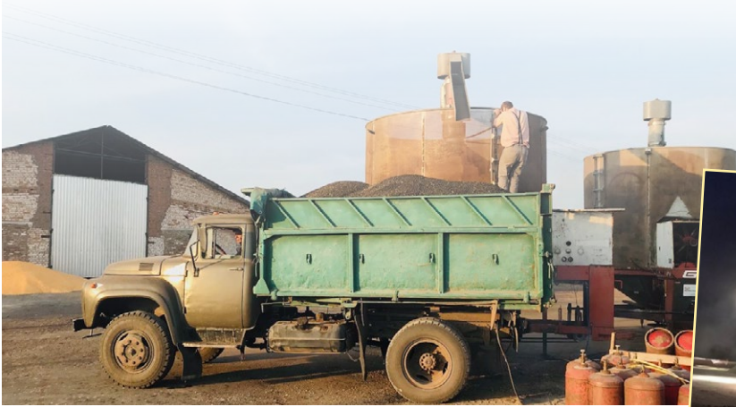
A farmer with a load of sunflower seeds awaits his turn at the dryer. The dryers run on propane, which is stored in the cylinders in the lower right.
