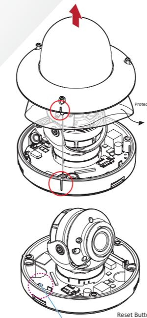
1 Detach the dome cover from the bottom case using the supplied torx before installing the camera.
