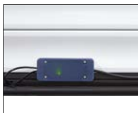
Wired optical sensor for safety
