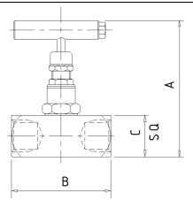
The Single Isolating Needle Valve is engineered for secure and dependable isolation, providing bubbletight shut-off. It features dynamic, self adjusting spindle seal to ensure long lasting performance across diverse applications.
