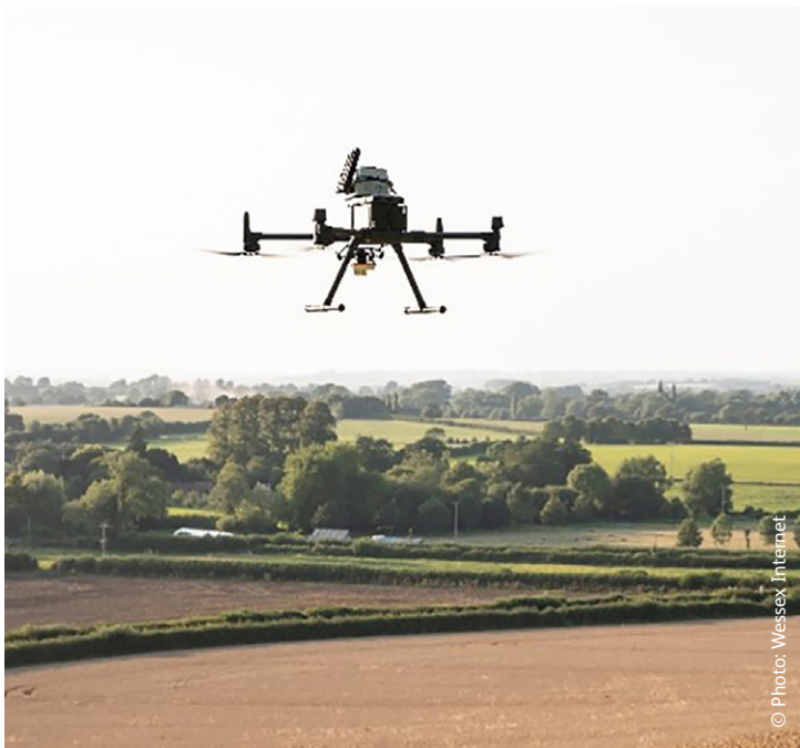
Figure 17: Drone fitted with 5G equipment flying at the trial farm. The 5G connection reduces image processing time from days to hours
