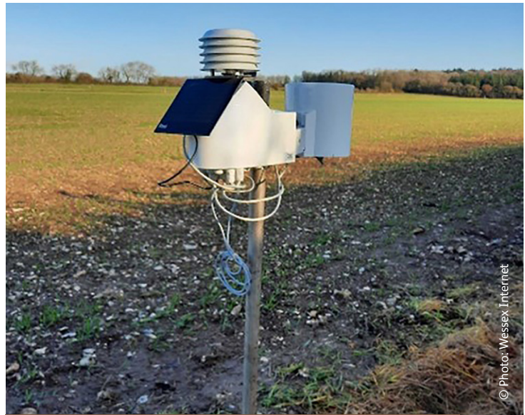
Figure 18: A 5G (NB-IoT) smart weather station. Although widely available, 4G coverage is limited and monthly costs are high. 5G (NB-IoT) will increase coverage and reduce costs
