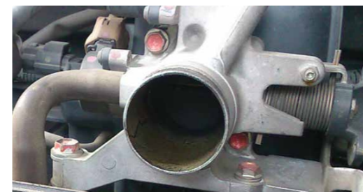
BEFORE (Throttle body condition after 60,000 km)
