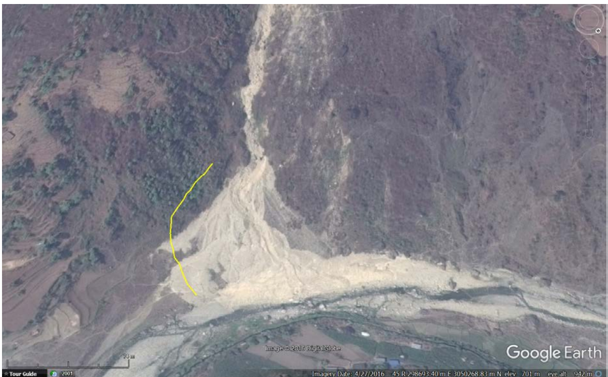
Figure 34. Base of landslide (yellow line) shown with homes and farmland impacted. Landslide manually identified by Durham University and the British Geological Society after the 2015 Nepal Earthquake. DigitalGlobe image from Google Earth.
