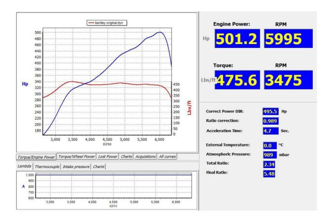
We then added 15ml of Oxytane directly into the fuel supply to give the desired balance of 1ml to 1 gallon of fuel and allowed the car to idle for 5 minutes giving the fuel enough time to mix. As this engine only runs on 4 cylinders when on idle we ran the car on the dynometer to see the results on the power and torque before testing for emissions. This allowed us to run the car over a few miles and enable all 8 cylinders to run the Oxytane treated fuel through the entire engine.
