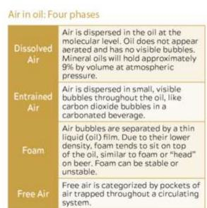
Entrained air can also affect the bulk modulus of hydraulic fluids, which in turn affects their compressibility. When hydraulic fluids become more compressible, the hydraulic fluid may become "spongy," causing unwanted compression and lack of precision hydraulic control.
