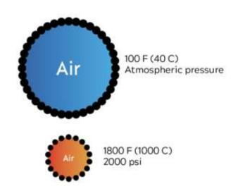
Micro-dieseling is caused by aeration and rapid pressure changes. It is most common in hydraulic systems and journal bearings.
