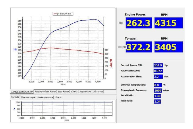
As the results show the car ran very close to the manufacturer's quoted figures. This is very good as the car was fitted with an automatic gearbox which usually lowers the dynometer power of a car by up to 10%.
