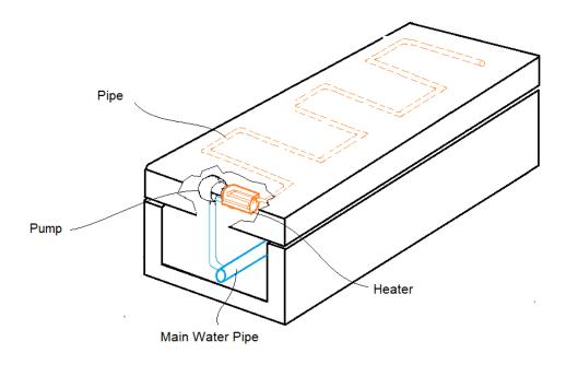
Water gets pumped from the Main Water Pipe by means of the Pump into the Heater where it is warmed and then goes into the Pipe through the Top Module to warm the surface of the Top Module.
