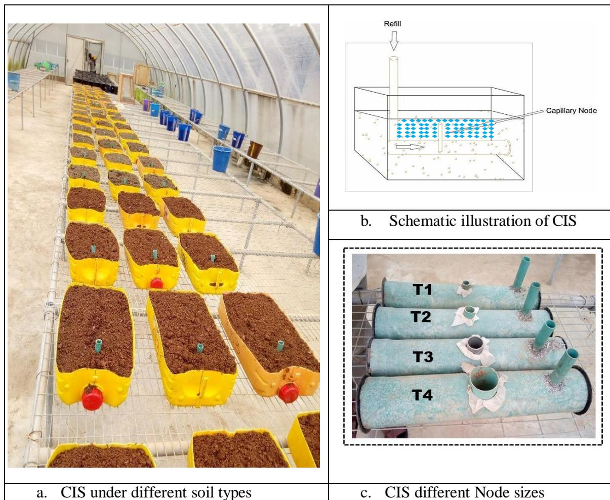
**Figure 2.** Capillary Irrigation system (CIS) setup and different capillary node sizes (T4: 50.8 mm, T3: 25.4 mm, T2: 19.1 mm, and T1: 12.7 mm diameter).
