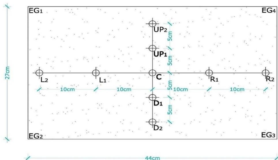
**Figure 3.** Designated points of monitoring soil moisture content in the capillary irrigation system setup. C= Center of the rectangular container, L1 and L2 = 10 cm and 20 cm left of C, R1 and R2 = 10 cm and 20cm right of C, D1 and D2 = 5 cm and 10 cm down of C, Up1 and Up2 = 5 cm and 10 cm away from C along the breadth respectively. EG1, EG2, EG3 and EG4 = vertexes of the rectangular container.
