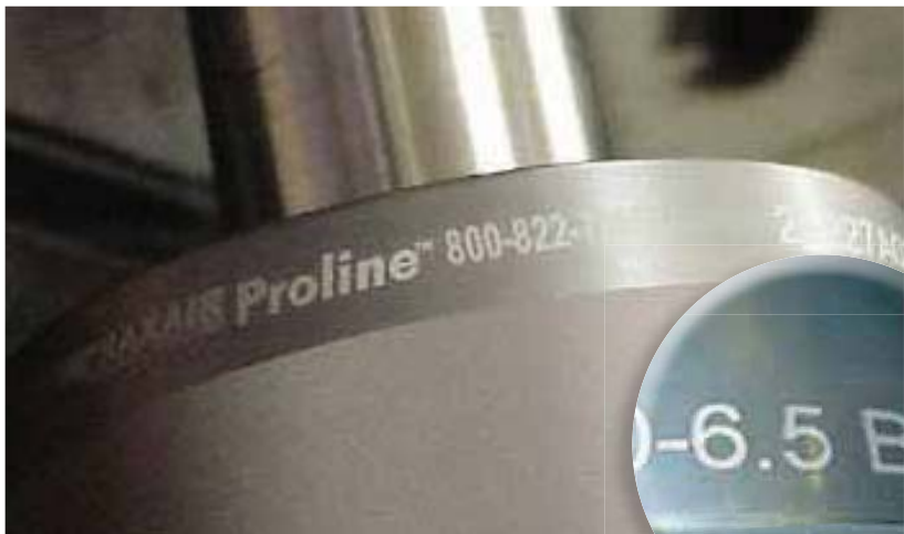
Roll marking technology provides unique identification data that is specific to each laser engraved ceramic anilox roll
