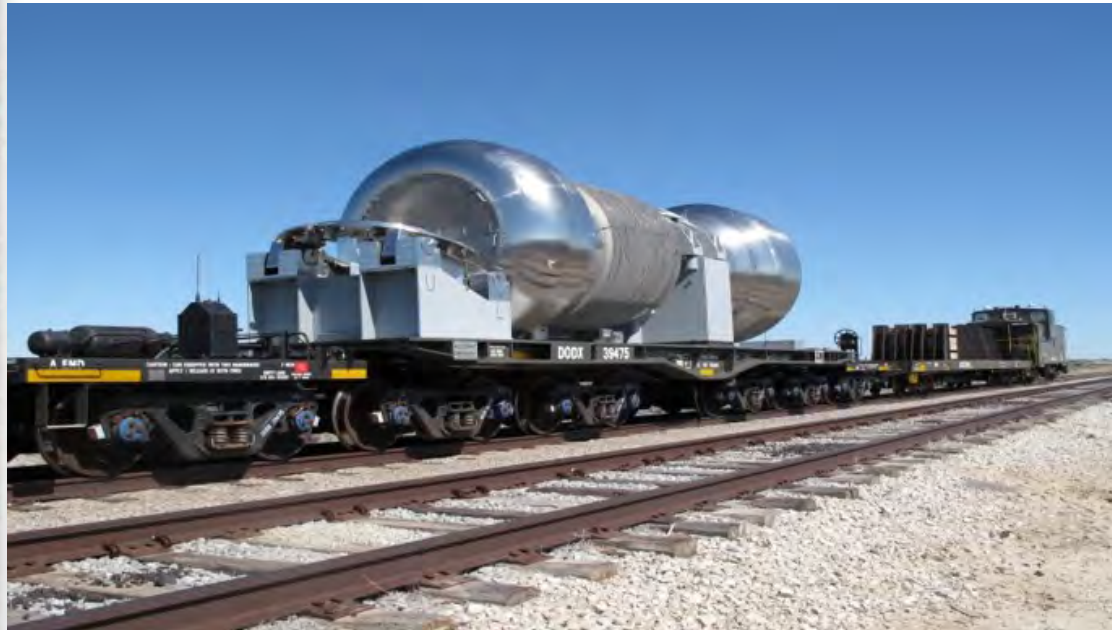
Transportation of a spent fuel cask by railcar. https://www.ornl.gov/division/rnsd/projects/spent-nuclear-fuel-transportation
