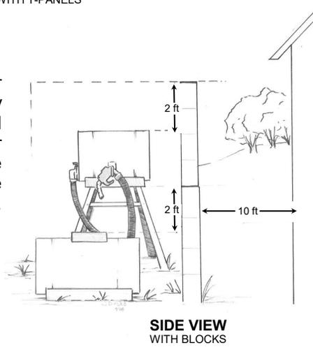
**CONCRETE T-PANEL OR BLOCK WALL (FILLED WITH CONCRETE)**
