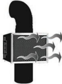
**Metal Pipe/Iron Pipe (Single-wall pipe used as a chimney):** Use of single-wall metal pipe, stovepipe, or iron pipe **will not** be permitted as a chimney for solid fuel-burning systems in dwellings or outbuildings.
