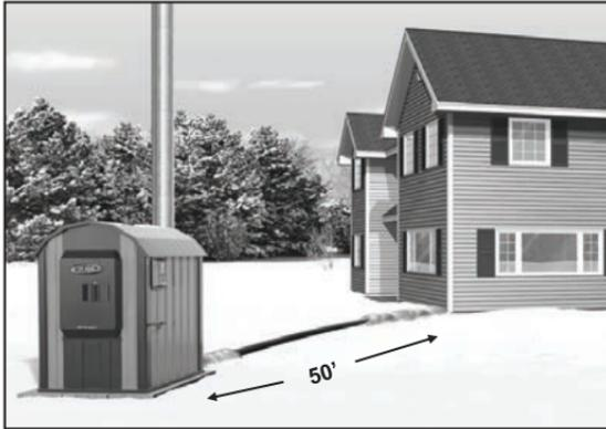
1. Outdoor hot water, wood-burning systems must be located 50 feet from any combustibles or structures. Spark arrester screens are required on the smoke stack.
