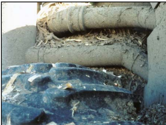
Crop residue accumulation around engine exhaust.
