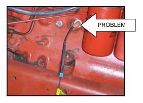
These cords should be inspected often and can be easily replaced. The loose end should be secured **to the tractor with zip ties** so movement does not put strain on the elbow. Twelve gauge extension cords should be used to supply power to the heater.
