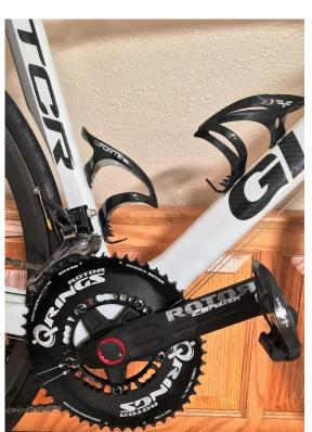
available inside a BB30 spindle than a BB86 spindle. Inside the spindle is where ROTOR inserts the electronics. But, for those that have a BB86 bottom bracket (example GIANT TCR ADVANCED), don't worry,
