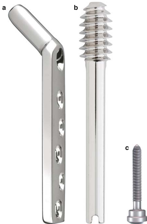
Fig. 6.50 Components of the dynamic hip screw (DHS). The main components are a side plate with a barrel (a) that accepts the sliding hip screw (b). The small compression screw (c) may be inserted at the completion of the procedure through the end of the barrel into the sliding screw for added compression. © Synthes, Inc. or its affiliates
