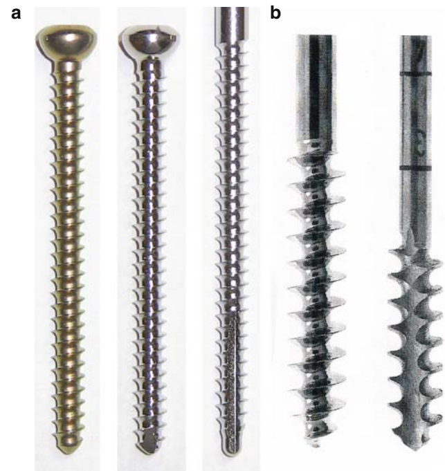
Fig. 6.15 Cortex screw and cortex tap (a), and cancellous screw and cancellous tap (b). The threads in the tap (right) are identical in shape to those in the screw but are sharp. The tap also has 3 longitudinal flutes near its tip. After the pilot hole is drilled, the tap is inserted in the hole to cut threads in the pilot hole identical to those in the screw. The screw can then be inserted in the threaded hole, without risk of bone fracture. Cortex screws are shown in titanium (left) and stainless steel (middle), and in non-self-tapping (left) and self-tapping (middle) varieties. ((b) from [2])
