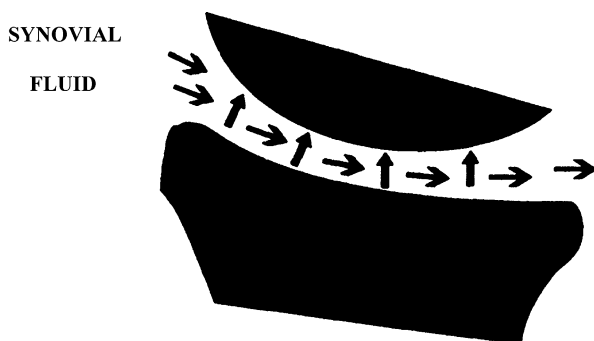
FIGURE 5.16. Hydrodynamic lubrication results in complete separation of the surfaces.
