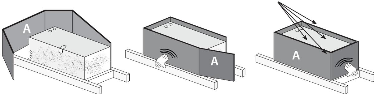
4. Set insulation in place by pressing firmly on all surfaces of the insulation that come in contact with the sides of the evaporator unit (see illustration).
