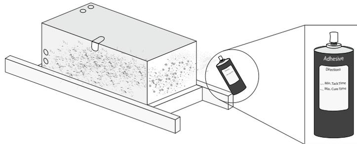
3. Wrap insulation piece (A) around the sides of the evaporator unit. Make sure the bottom edge of the insulation is flush with the top edge of the mounting bracket (see illustration).
