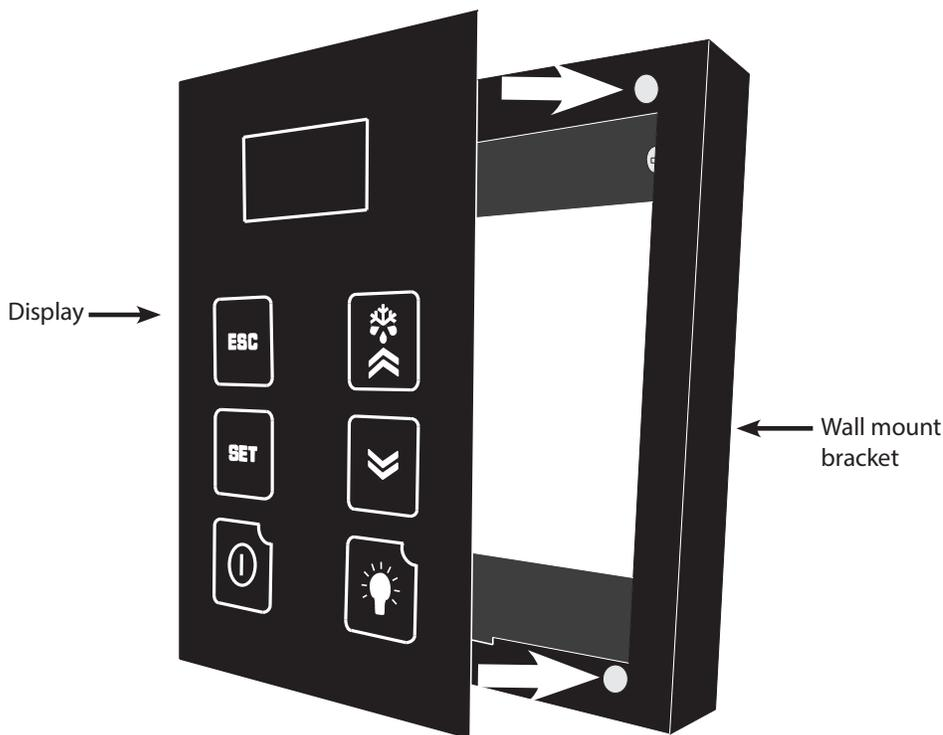
5. Place the display on the wall mount bracket as shown, attaching the back of the display panel to the magnets on the mounting bracket. Make sure that the alignment tab on the back of the display panel sits in the notch on the bottom of the bracket.
