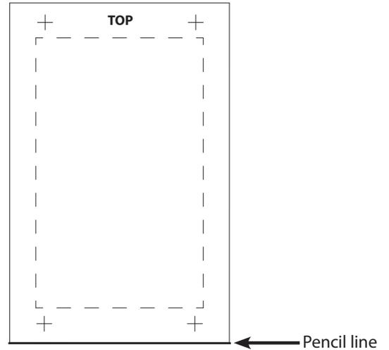
3. Use a  $\frac{5}{16}$ " drill bit to drill a hole in the center of each cross (+).
