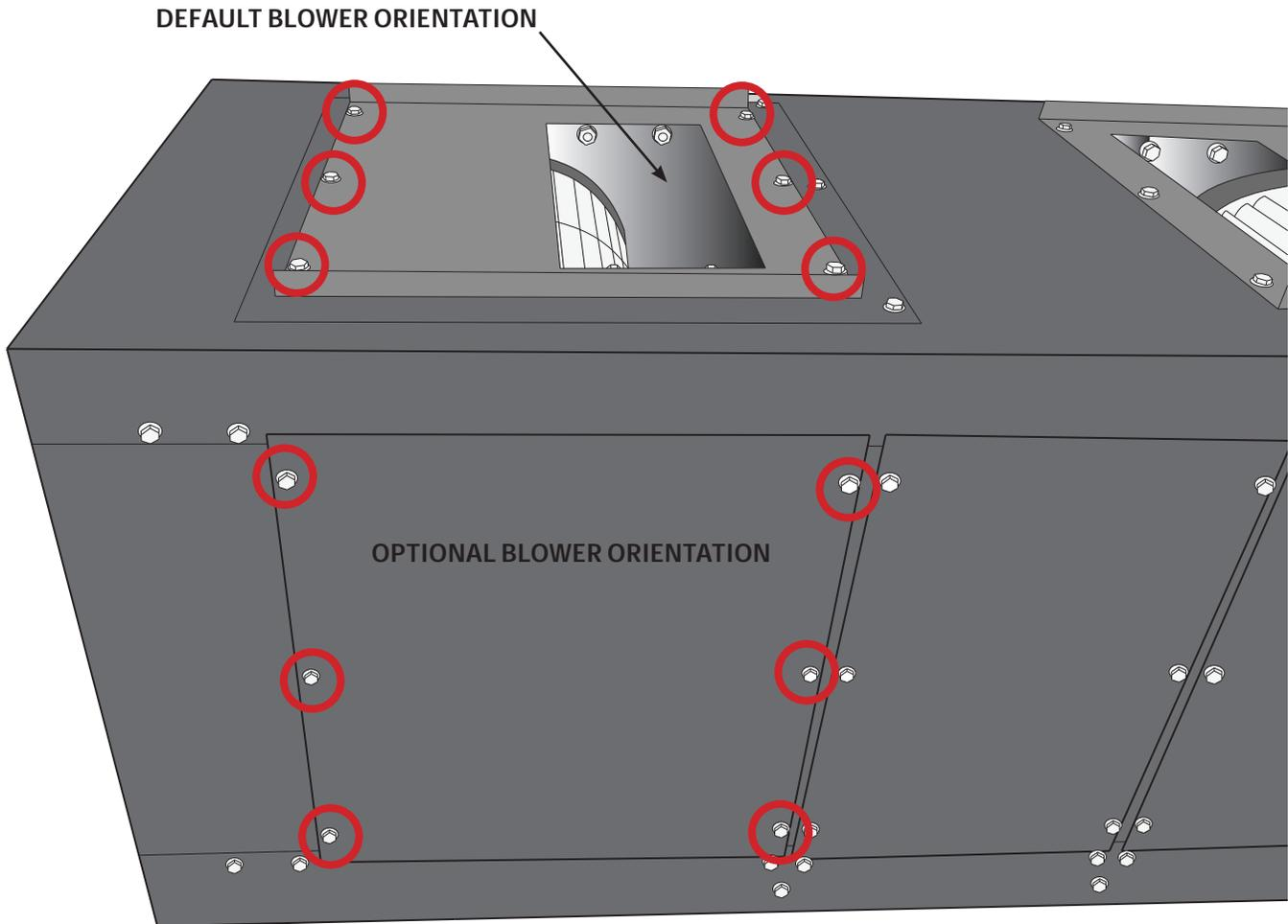
3. To reorient the blower(s), first remove the screws securing the supply panels on the top and preferred side of the unit (as shown above). Remove the panels.
