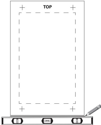
2. Peel the backing off the template and stick it to the wall, aligning the bottom edge with the line drawn in Step 1.
