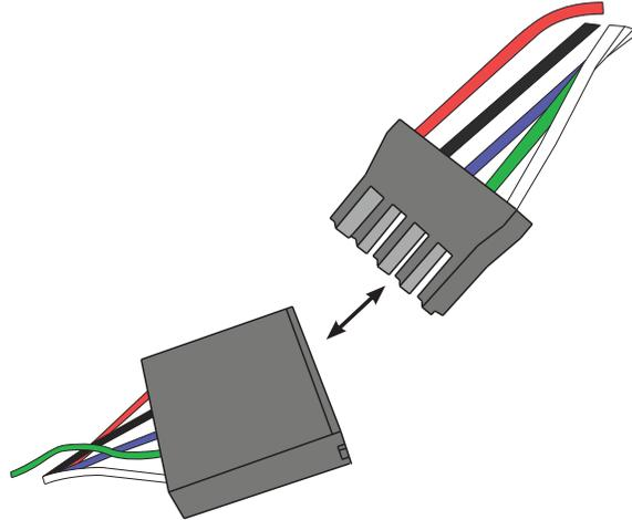
5. Remove the blower from its current location and connect the Molex connector. Ensure that the blower remains in the orientation shown.
