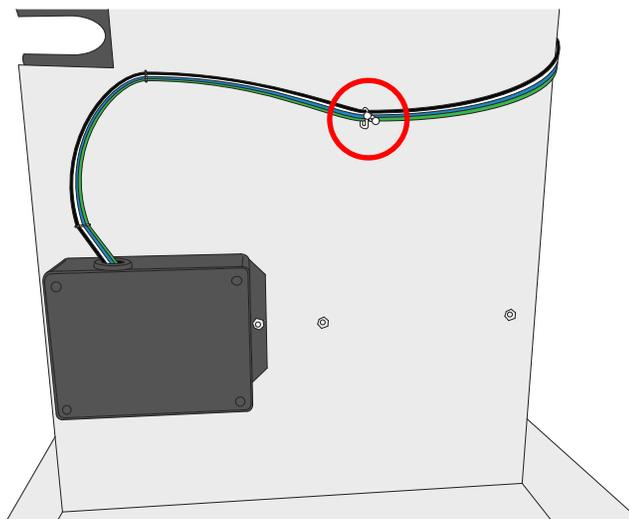
4. Resecure the wires using the twist clip.
