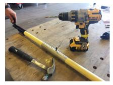
Insert the 3 supplied roll pins, leaving the corresponding hole open so the R.E.A.C.H. can wrap around the sleeve when in the stored position.
