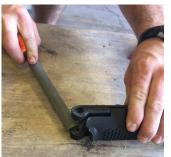
To customize the fit of the R.E.A.C.H. between the sleeve and the handle when wrapped around the shaft, a small amount of filing may be required. The R.E.A.C.H. will snap when fully engaged open and closed.
