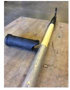
Decide the orientation of the handle (the position you would like to use it when perpendicular to the pole) before drilling
