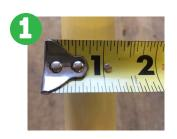
Measure your pole. The handle and sleeve are specifically engineered for use on a standard non-tapered 1.25" pole. (a fire industry standard)
