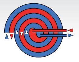
The hot flow enters in the center of the heat exchanger and exit to the outside. The cold flow is from the periphery to the center : counter- current flow effect.
