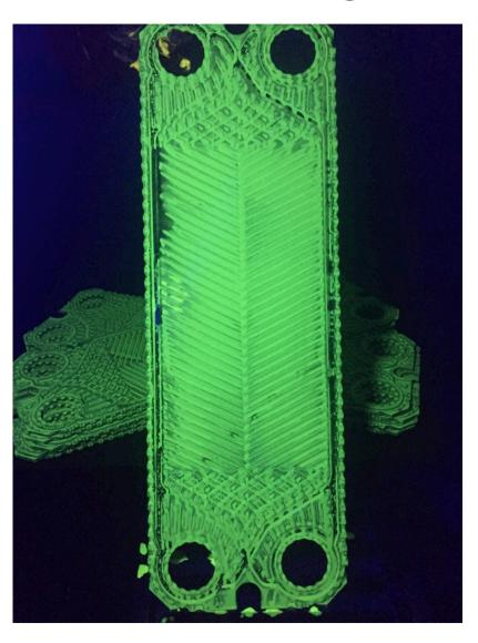
We use special UV equipment to spot all cracks and pinholes
