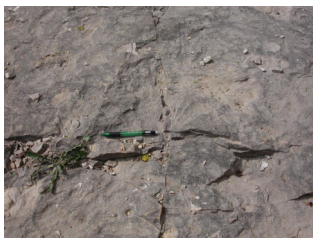
Bedrock surface (~623 ft above MSL). The pencil is along a joint trending N44W. The perpendicular joint, just to the right of the pencil is trending N34E.
