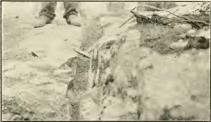
A typical silver-cobalt vein, outcrop on Coniagas, Cobalt. The head of the hammer shows the width.
