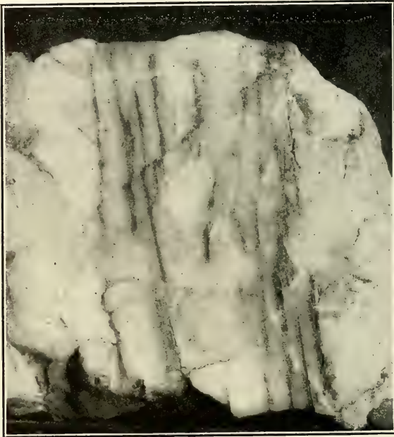
Streaked ore from the Jupiter mine, Porcupine. The dark lines are tourmaline; the quartz is much crushed and contains visible gold.
