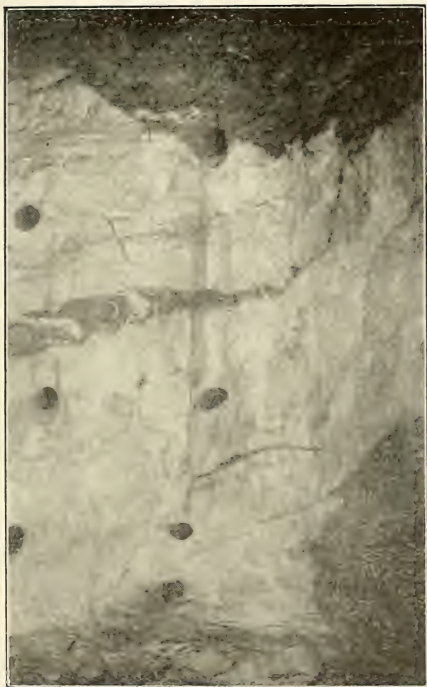
Quartz vein on 100-foot level, McManney mine. The dark spots are drill holes.
