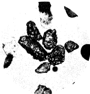
FIGURE 62, B Garnet grains from the Miner's Castle member. Sample from drill-hole core from Alger County. X63.
