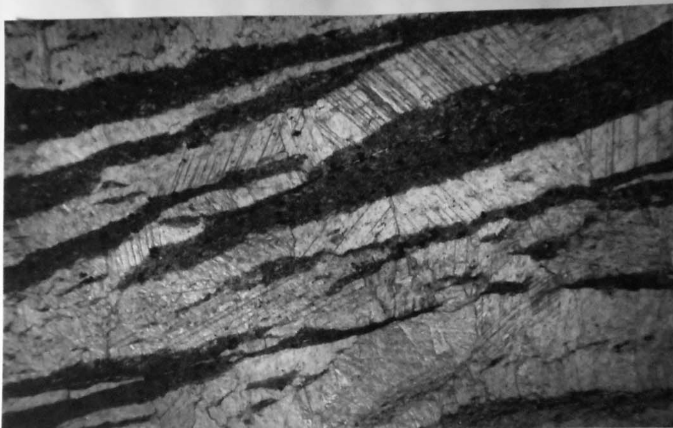
Figure 29. Microscopic appearance of carbonate-mineralized fault material in slates (field of view is approx. 6 mm.; plane-polarized light).
