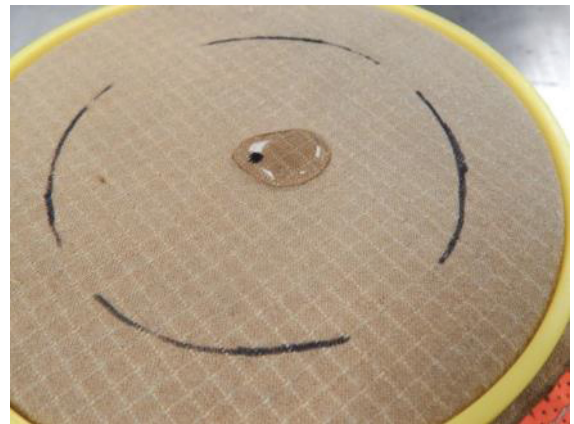
Figure 6: Measurement of horizontal wicking distance
