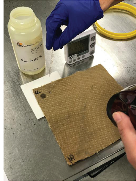
Figure 4: Oil repellency test set up
