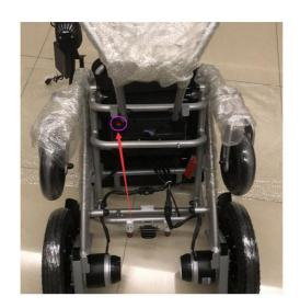
(When this switch is turned on, the wheelchair will stop working but will charge. This is done to protect the user from accidental operation during charging. Increase security.And the charger will automatically stop working after the battery is fully charged to prevent the battery from being overcharged. Has automatic power off function.)
