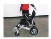
3. Install the controller: Insert one end of the extension tube of the controller into the ring hole of the handrail tube on the right side of the vehicle, then tighten the plum blossom knob; push the power cable backwards to reach the straight state. (pictured)
